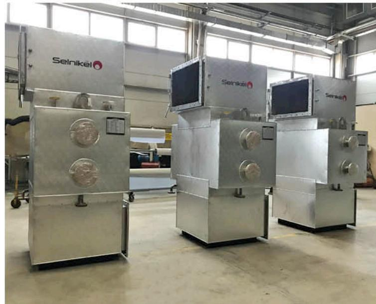
The thermal design of the economiser is performed in accordance with the given parameters of exhaust gas volume and temperature, feedwater volume - temperature and the required flue gas temperature downstream of the economiser. The philosophy of economizer is the same as that of air preheater.
